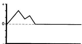
Figure 36c DCO pitch modulated by DCO env; pitch velocity = 00
