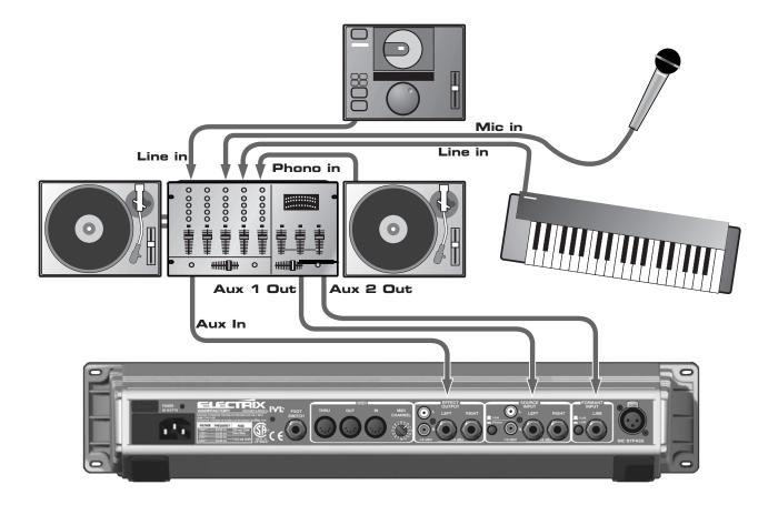
This is a simple setup for stereo processing of the entire mix. Selecting the Mic or the Auto settings for the formant input will provide plenty of sonic possibilities. Use this setup only after you have explored all the sonic possibilities of WarpFactory because cueing is not possible. The cueing limitation can be minimized by bringing in the effect gradually with WarpFactorys mix control and then making any adjustments from there.
